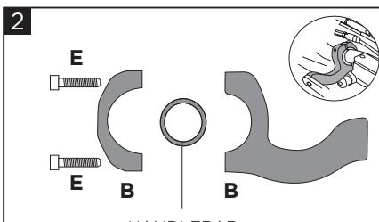
**Mount the bracket (B) on the handlebar using screws (E).**
