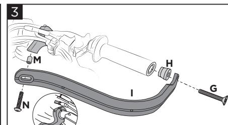
**Fix the bar (I) to the handlebar using the spacer (H) and the screw (G) as shown in the figure. Fix the bar to the bracket using the bushing (M) and the screw (N).**
