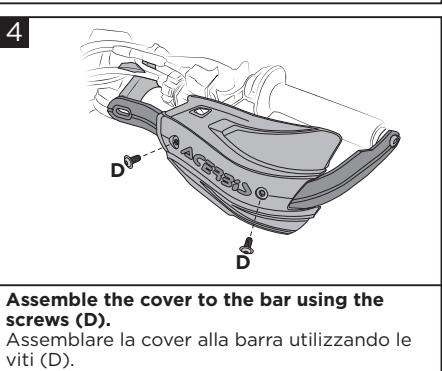
**Assemble the cover to the bar using the screws (D).**
